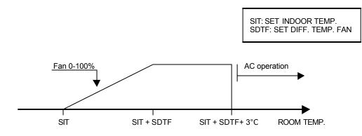
When the outdoor temperature is below SET INDOOR TEMP. (SIT) the fan operates to cool the room controlled by 3-10 V analog signal (approx. 80-230Vac) across set working range according to figure above. Intake air damper is open and mixing damper is regulated depending upon outdoor temperature (see 3,1).
