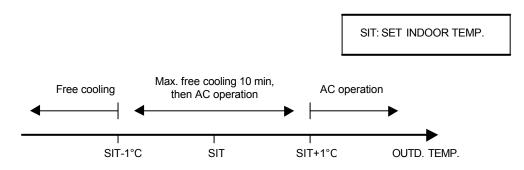
When the outdoor temperature is below or equal to SET INDOOR TEMP. -1°C free cooling is in operation. The outdoor air temperature contains enough cooling capacity to maintain radio base station climate at the desired temperature.
